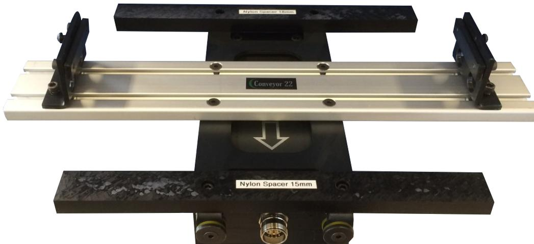
2 Nylon Spacers mounted together with Aluminum Bar and tray attachment on Black Line ECS-121 conveyor
